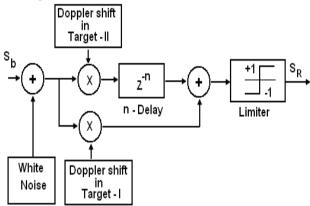
Fig. 8 Target Model When Two Targets are at n-SPDA.
